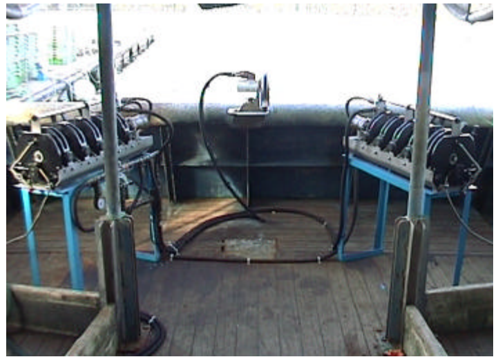
Figure 3 Hydraulic Tuna Trolling Gurdies & Stern Puller
